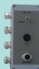
P-711 Engine Room Station
